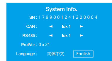
◆ In the system information page, the serial number, communication protocol, protocol version and language will be displayed. When you need to communicate with different inverters, you can choose the corresponding communication protocol.
